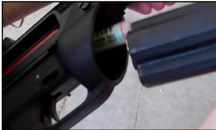
When the magazine was able to be properly inserted into the weapon, a fail to feed malfunction then became an issue. The magazine is required to be manually rotated after each four shot magazine tube has been expended and the bolt automatically locks in the rearward position. When the magazine cylinder was rotated to the next tube, the subsequent round would
