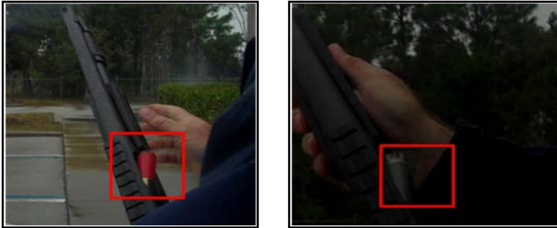
Figure 6. Stove Pipe Malfunction
