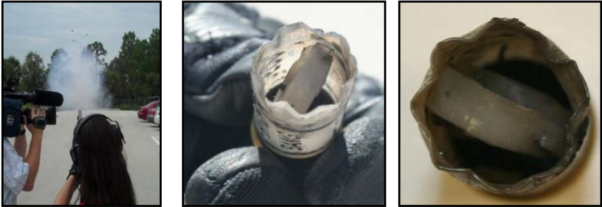
Figure 7. Chambered Mmunition Detonation
