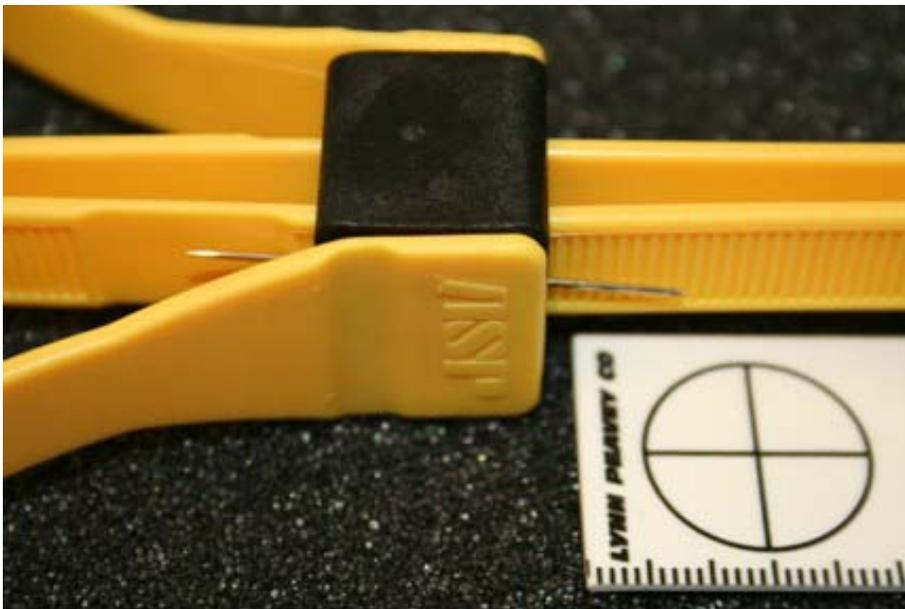
Additionally, the Tri-Fold failed a basic durability test as it was possible for one of the investigators to actually break free using only brute force. As shown below, one locking mechanism separated from the rest of the restraint. However, the second locking mechanism also failed by allowing the strand to slide through the pawl.
