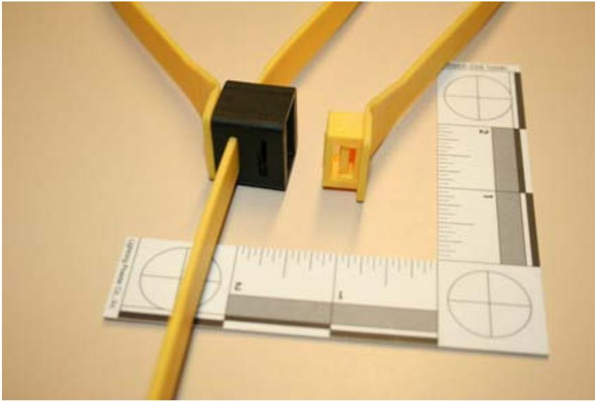
Given the dynamic nature of this failure, we replicated this test by applying the restraints in both the front and the rear of the tester. Each time, the tester was able to cause the restraint to fail by pulling the strands in opposite directions. The locking mechanism appeared to be unable to maintain traction on the “teeth” of the ratchet and the strand was able to slide free.
