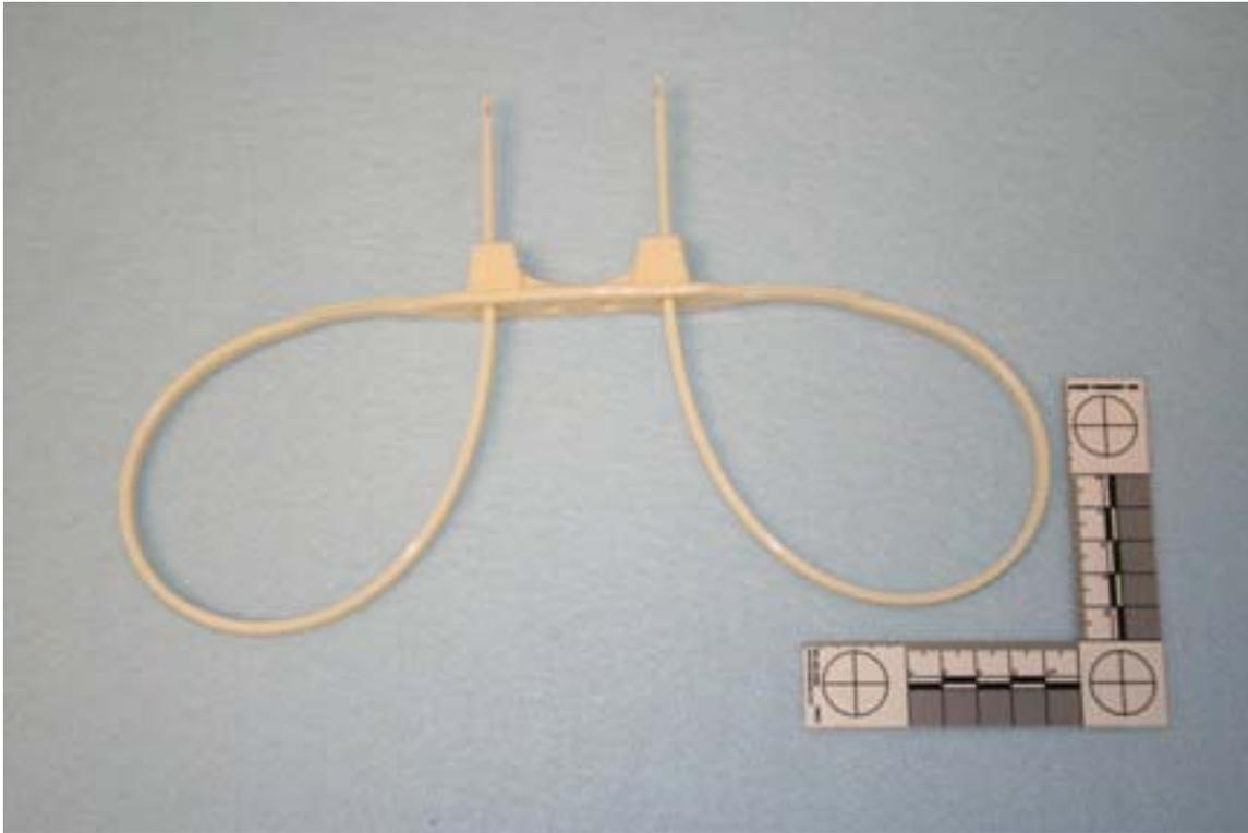
The Tuff Cuff Disposable Double Restraint is comprised of a double nylon material with a tensile strength of 400lbs and a cost of \$1.26. This restraint has a double locking system that prevents the restraint from over tightening on the individual. The Tuff Cuff works by inserting the strands into the pawl, and then pulling the strands to tighten them securing the individual.
