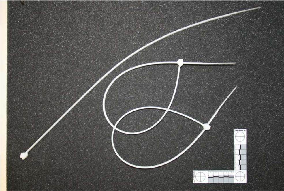
The Flex Cuff disposable restraint is comprised of a strong nylon material with a tensile strength of 300lbs and costs \$1.15. This restraint has a unique strength barb system which is a small piece of metal within the pawl making the restraint more difficult to escape. The Flex Cuff functions by looping two strands together and feeding the strands into the pawl.
