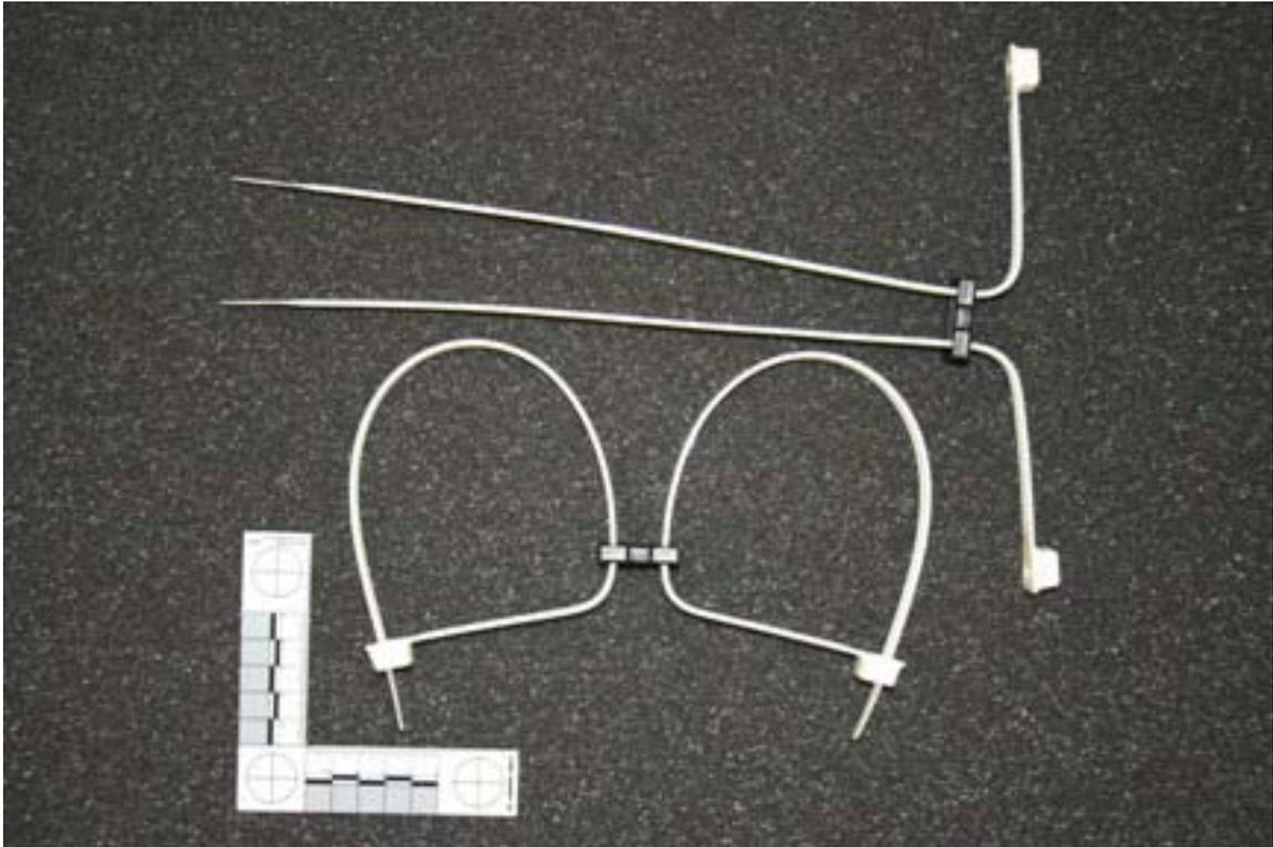
The EZ Cuff Model 500D Double Loop restraint is comprised of lightweight nylon material. The restraint has a tensile strength of 600lbs and a weight of 24 grams with a cost of \$1.34. Each strand is secured by a connecting bridge and functions by inserting the strands into the pawls and pulling tightly to secure an individual.
