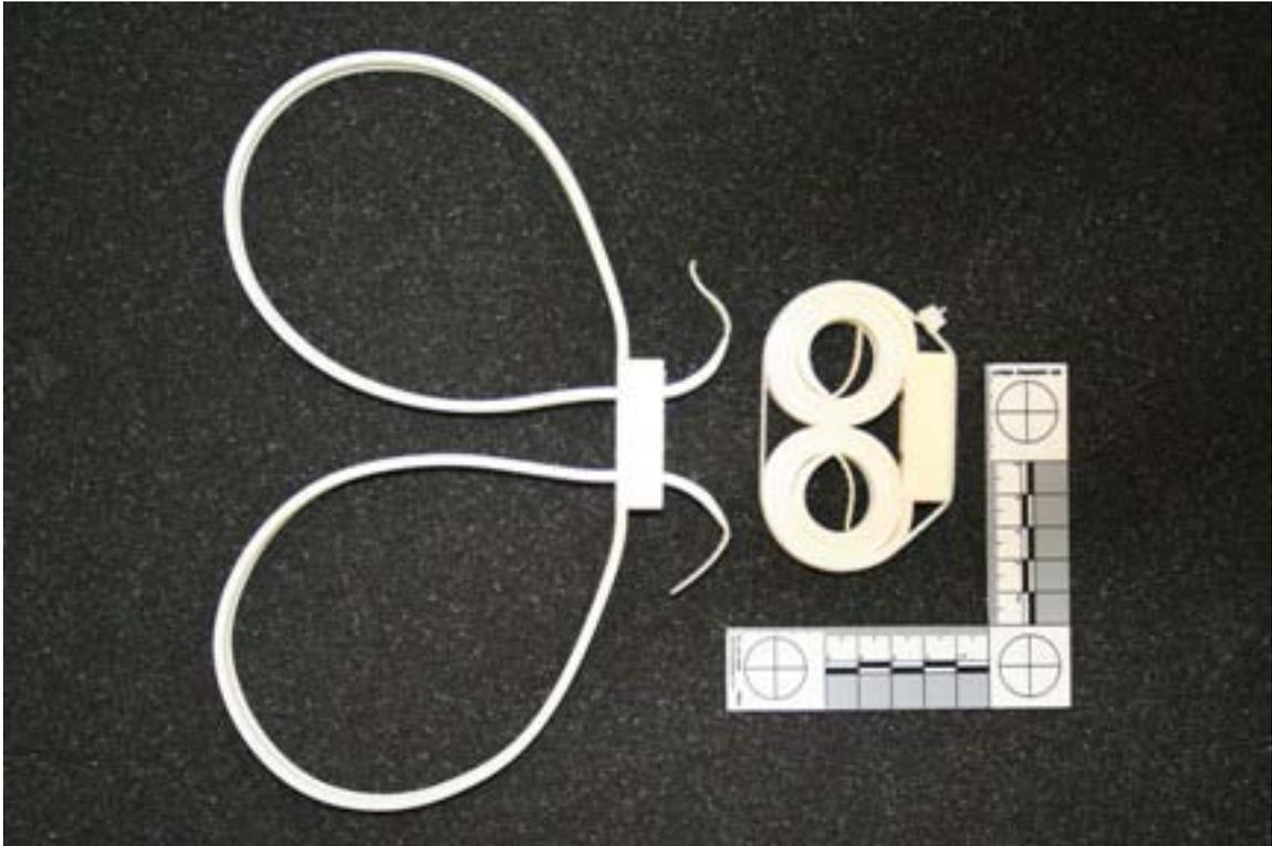
The Monadnock Double Cuff and the Monadnock Compact Double Cuff are comprised of a lightweight nylon material. Both have a tensile strength of over 400lbs and weigh 34 grams. The Monadnock Double Cuff costs \$1.46 while the compact version costs \$1.99. Each version functions by inserting the strands through the pawl and then pulling the strands tightly to secure. The compact version is packaged with the straps wound tightly inward and banded together for easy concealment and carry.
