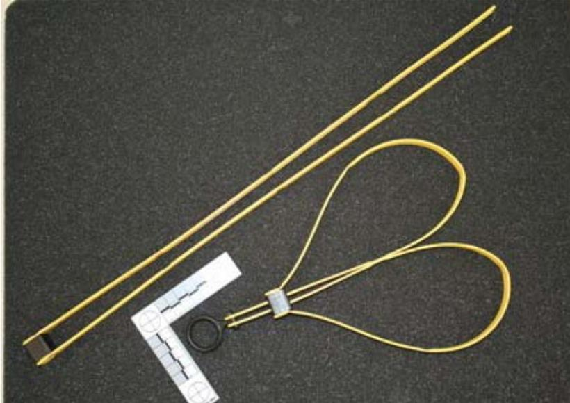
The ASP Tri-Fold disposable restraint is a compact and easy to carry device composed of a high strength polymer weighing 36 grams with an average cost of \$2.83. The restraint functions by inserting the strands into the pawl and then pulling the strands tightly to secure an individual. A ring allows both strands to be tightened simultaneously by pulling rapidly.
