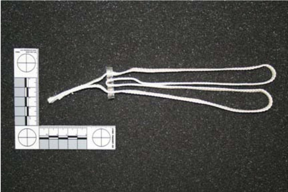
The Tuff Tie Hand restraint is comprised of braided nylon cords while the pawl is made of a polycarbonate locking block. The tensile strength is 500lbs with a weight of 8 grams and costs a \$1.30. The restraint comes fully assembled and the pig tail designed cord allows for a knot to be tied once the restraint is locked for added security.
