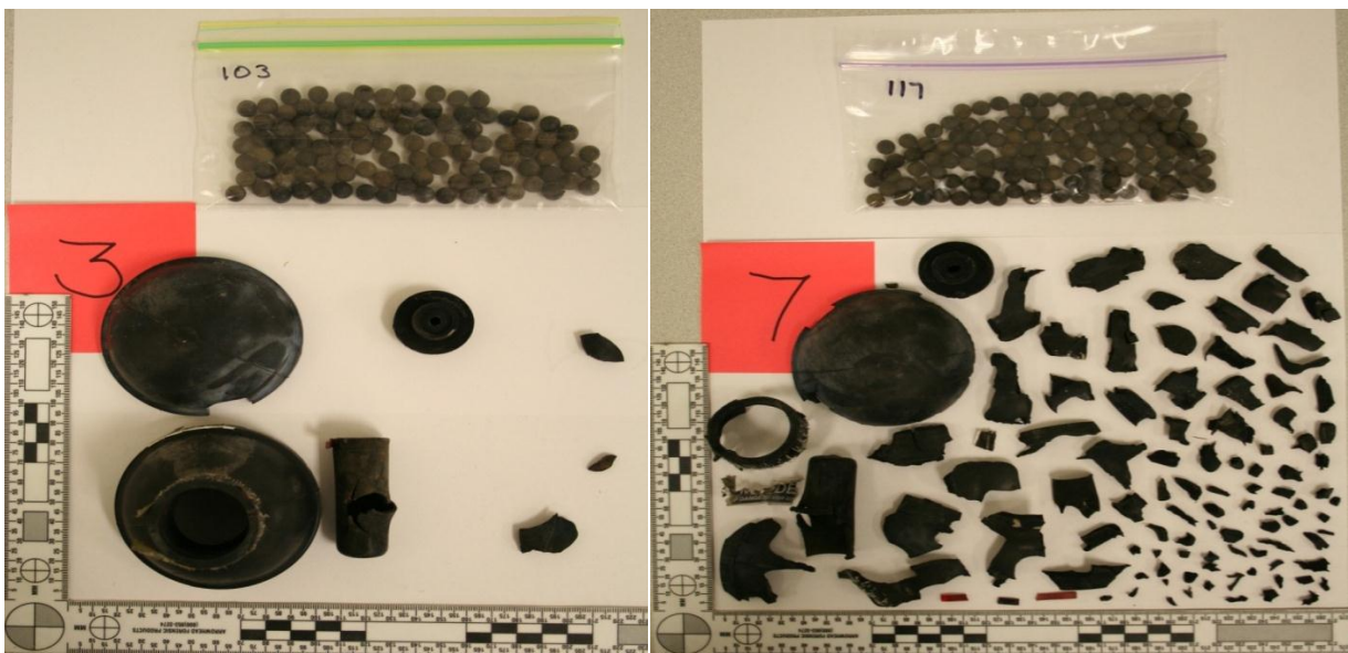
Figure 3. Different Fragmentation in Two Stingball Grenades
