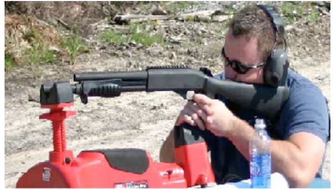
FIG. 3—Tester firing from a fixed platform position. The bench rest is used to reduce human error while aiming.
