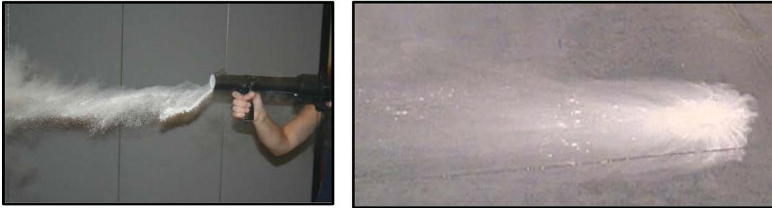
After malfunctioning shots were fired, the powder covered the gun, the cartridge and the shooter’s hand, arm and fingers. *Figure 7* (left photo) illustrates how the shooter’s hand was covered in the inert powder after cartridge malfunctions. The center photo illustrates the cartridge and the gun covered in the powder due to a malfunction. The photo on the right shows more powder covering the gun and the shooter’s hand.
