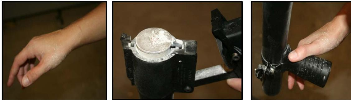
After a test shot that produced the visible clumps and large amounts of excess powder, a sample was collected and weighed. In this single instance, 13.04 grams was dumped from the gun (representing approximately 36% of the payload) and is equivalent to approximately five PepperBall® projectiles (see WERI report “PepperBall® SA-4 Launcher™ Accuracy Study” for more information on PepperBall®).
