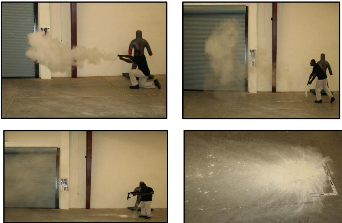
*Figure 2* illustrates the sequence of events in a malfunctioning muzzle blast cartridge deployment. The discharge of the cartridge is shown in the first photograph. As the launcher is lowered, a substantial amount of payload is seen falling from the barrel (second photo). The last two photos show the final amount of payload that was released as the breach of the launcher was opened.
