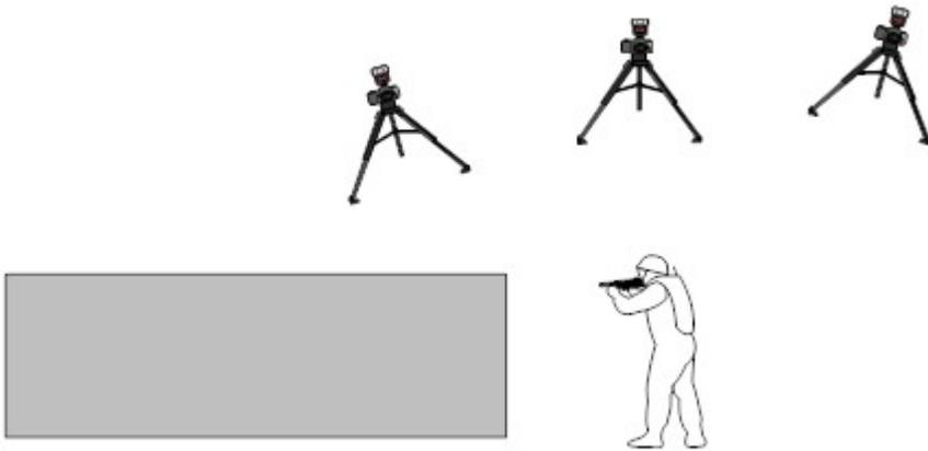
All staff affiliated with the study and the operator was certified in less lethal munitions. Four rounds of an individual brand were loaded into the tubular magazine of the weapon. The operator then fired the first round and unsuccessfully attempted to pull the trigger to cycle remaining rounds. The operator was then required to manually cycle through the remaining rounds.
