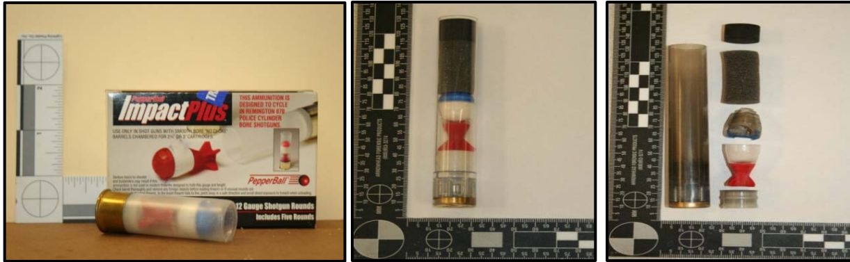
Figure 2. SA-4 Munitions Components
