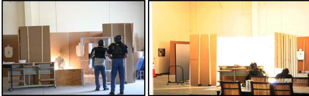
The grenade was remotely detonated while attached to the bang pole (which was placed on the ground) and cardboard panels were marked where grenade pieces and rubber balls penetrated the surface of the cardboard. The data from each deployment was mapped onto a data collection form and collated for later analysis. Photographs and videos of testing made it possible to reconstruct the results of each deployment.
