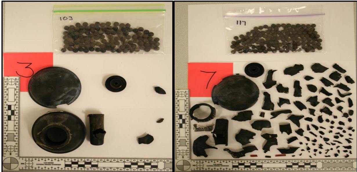
Some grenades fragmented into a few large pieces while others fragmented into dozens of smaller pieces. The researchers categorized shrapnel from the grenades into three size groupings, 0-20mm, 21-40mm and greater than 40mm. As shown in Table 3, the majority of the shrapnel fell into the smallest category.
